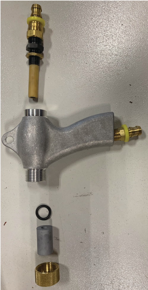
Expanded view of blast gun.
